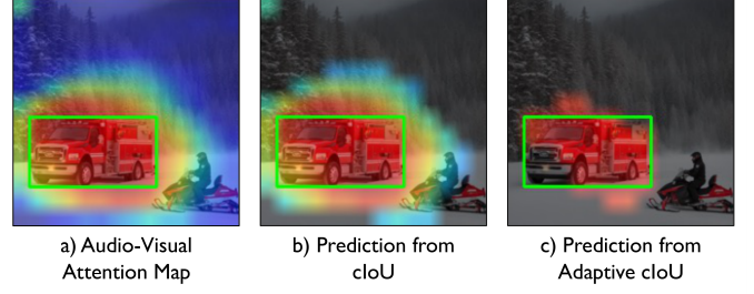
Fig. 5. Qualitative comparison of cIoU and Adaptive cIoU in the area used for quantitative analysis. (a), (b), and (c) depict the audio-visual attention map results, the predicted area from the perspective of cIoU, and the perspective of Adaptive cIoU, respectively. The gray color signifies the background. The ground truth bounding box is annotated in green. Although the localization area successfully covers the bounding box in (b), the sample cannot be considered correct since the prediction is much larger than the ground truth. However, Adaptive cIoU better evaluates model performance with small ground truth sizes.
